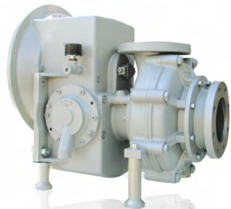
TYPE: RUBERG EUROLINE type: single-stage material: bronze / aluminum* output: 2 000 - 4 000 l/min - 10 bar
